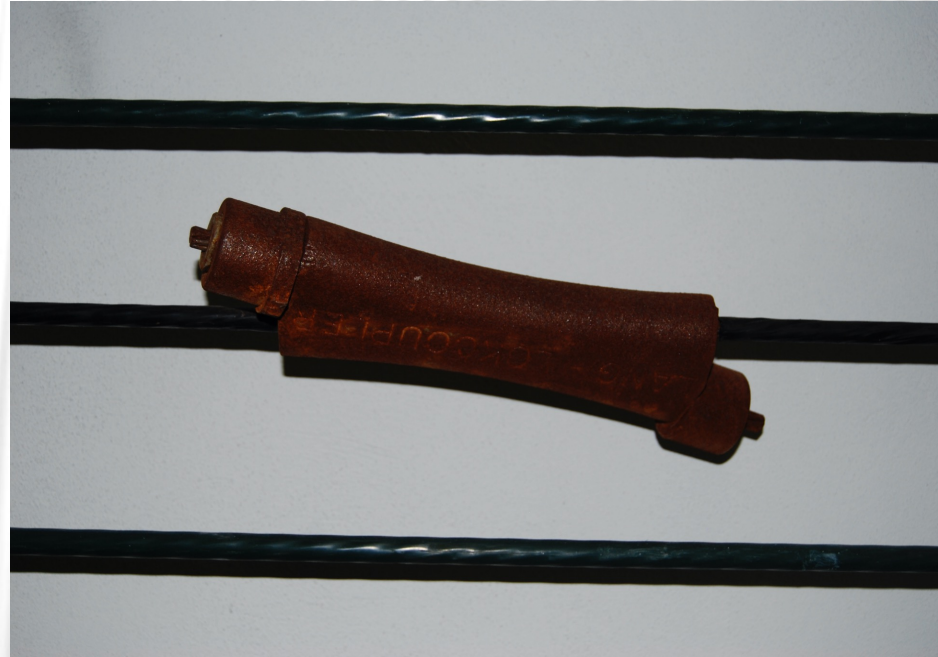
Examples of corroded structural cable anchor and splice.
