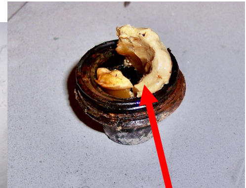
Opaque grease is a sign of water intrusion
