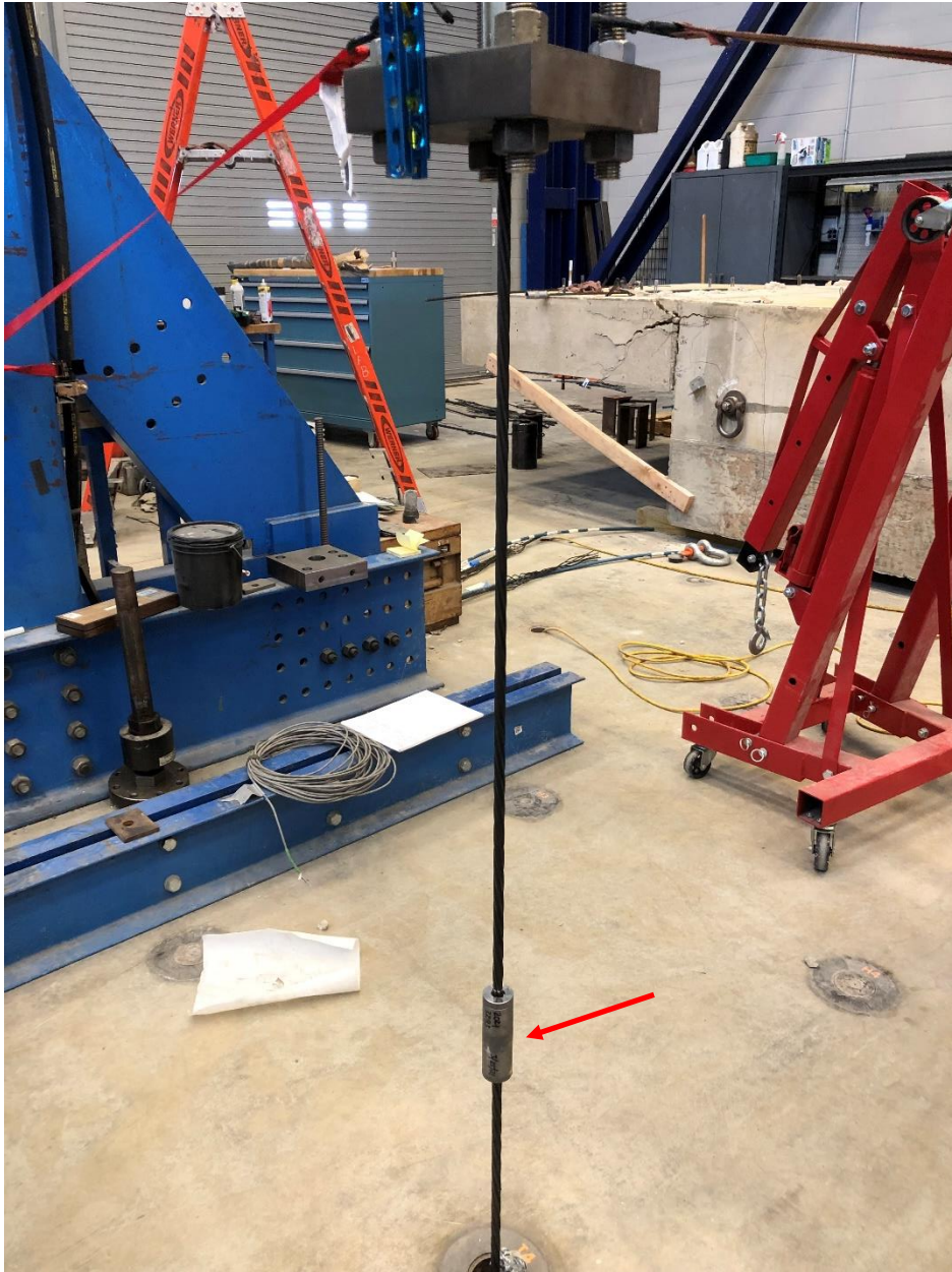
Figure 2. Splice Coupler – 0.5-in fatigue sample
