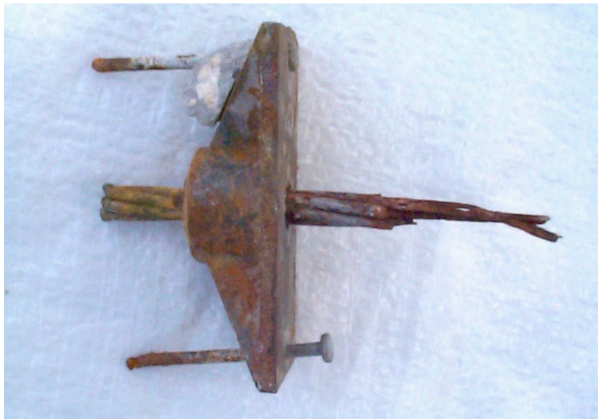
Photo: Tendon end that shows cable corrosion due to water intrusion into the cable sheathing.
