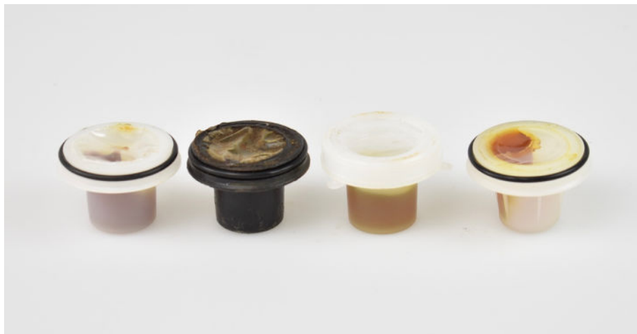
Image 11: Examples of grease caps from several different encapsulated anchor systems.
