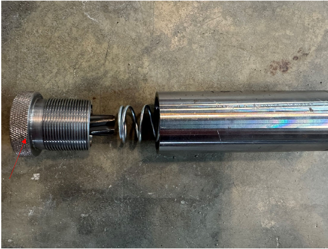
Figure 1. SC1 Splice Coupler showing one end with strand and spring used to hold wedges in place.
