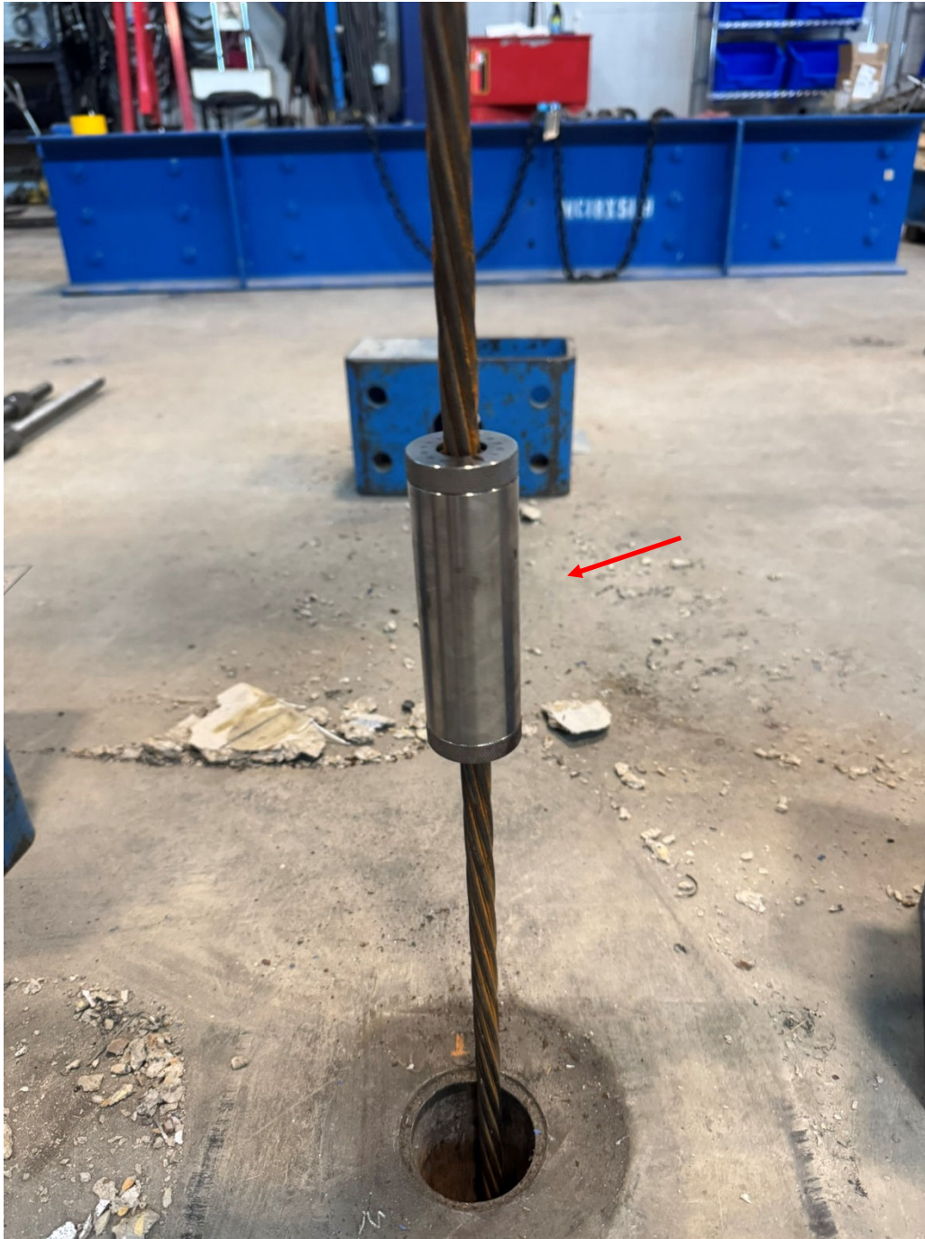
Figure 2. SC1 Splice Coupler fatigue sample with top end anchored to hydraulic actuator and bottom end bearing on structural floor soffit below.
